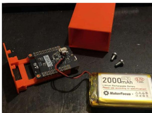
Figura 45 - Invólucro plástico projetado para comportar Lilygo TTGO T7 ESP32 junto a uma bateria recarregável. Fonte: [https://media.printables.com/media/prints/149999/images/1412160\\_4b667954-40ee-40f8-902f-aea7b9a8bb23/thumbs/inside/1600x1200/jpeg/img\\_8133.webp](https://media.printables.com/media/prints/149999/images/1412160_4b667954-40ee-40f8-902f-aea7b9a8bb23/thumbs/inside/1600x1200/jpeg/img_8133.webp)
